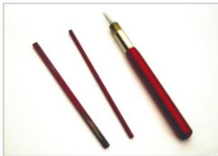
Figure 2. A sapphire burnisher and two Degusset stones.
