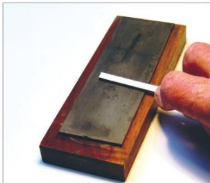
Figure 8. A pivot burnisher being sharpened on a fine diamond block.
