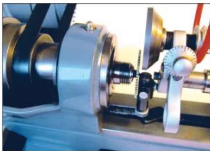
Figures 12 and 13. A burnishing tool by Bergeon.
