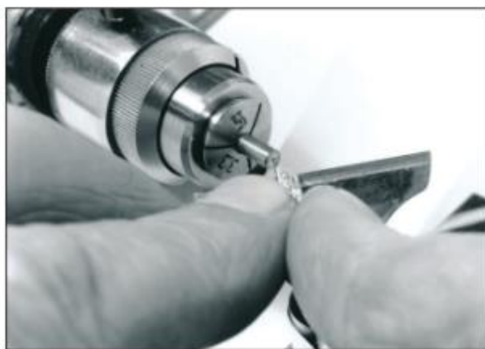
Figure 23. A centre being cut with the graver.
