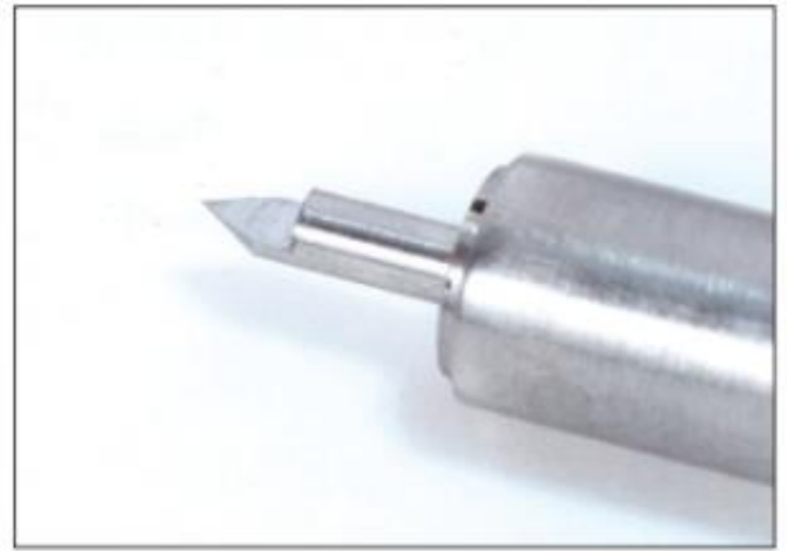
Figure 25. A homemade 'D' bit centre drill.
