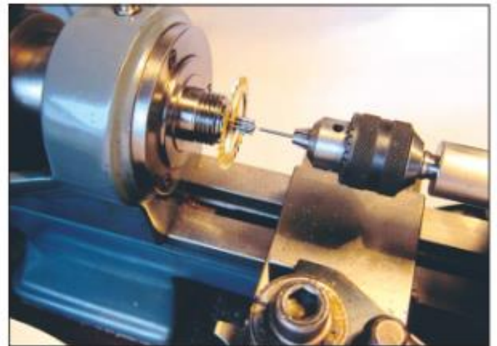
Figure 27. An escape wheel and arbor, held in a good collet and drilled from the tailstock.
