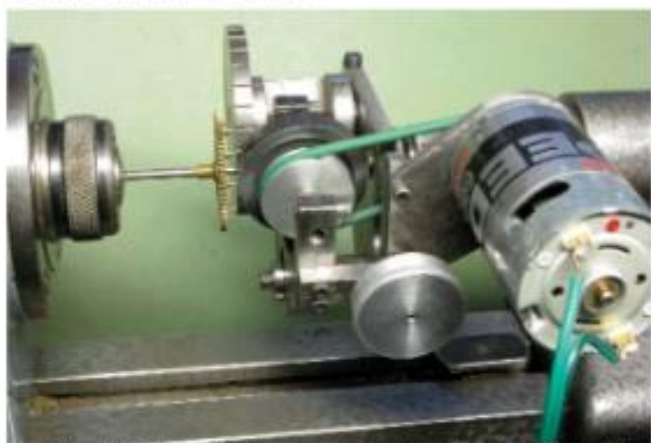
2. A clock striking arbor having a pivot burnished in a Schaublin 70 precision lathe.
