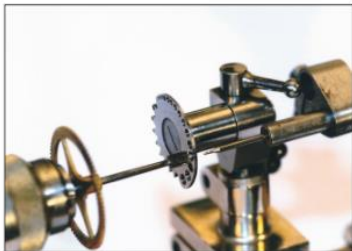
Figure 30. The drill plate mounted on the tee rest base.
