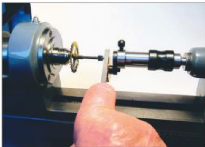
Figures 4A and 4B. The set-up for re-finishing the pivot in the Schaublin 70 lathe.
