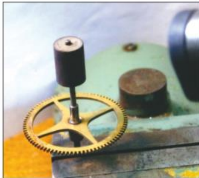
Figure 39. When softened, the arbor should be a nice blue.
