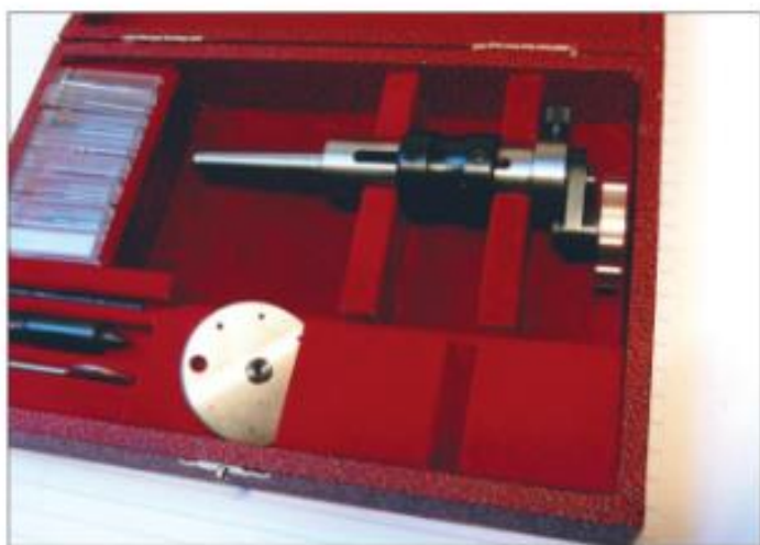
Figure 4C. The complete tool in a fitted case with drills and drill plate.
