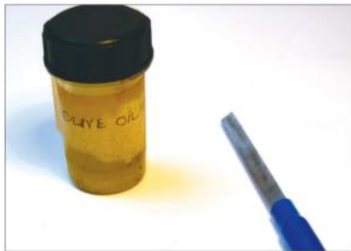
Figure 7. A lubricant is used on the burnisher.
