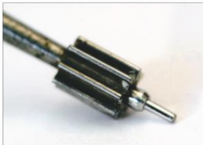
Figure 9. A completed pivot.
