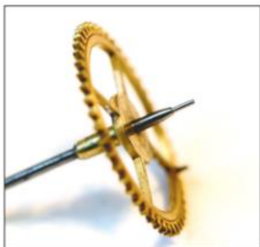
Figure 36. The blued pivot steel in position.
