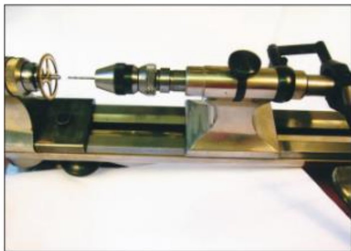
Figure 31. The lever feed tailstock on the 8mm Boley & Leinen precision watchmakers' lathe.
