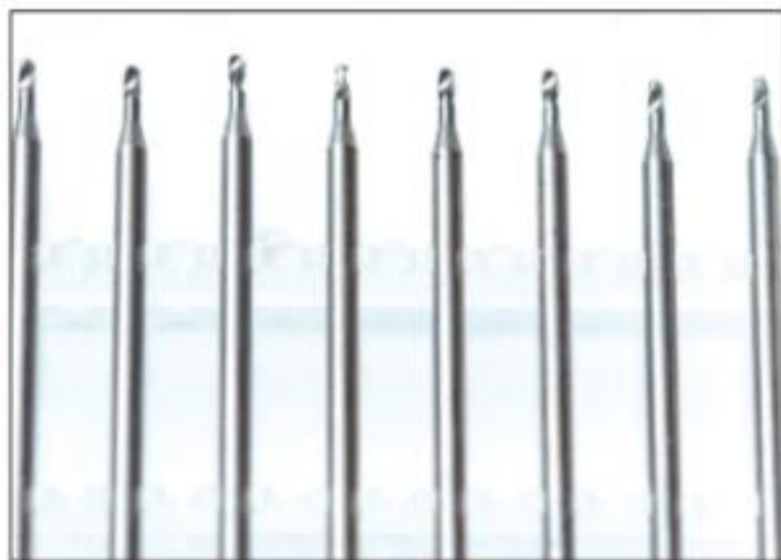
Figure 21. Another range of Fenn drills are the spotting drills.
